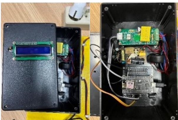
Fig. 4. (a) 16x2 LCD installation, (b) SiMONDE component placement in the packaging box
