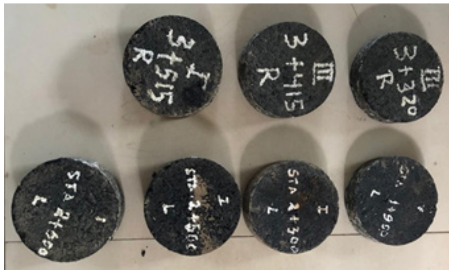
Gambar 10. Sampel Latasir Hasil Core drill
